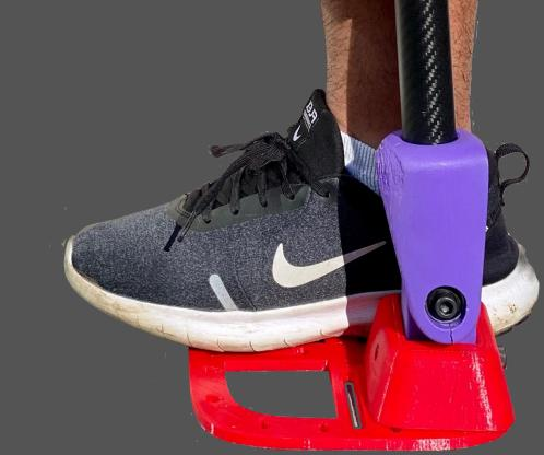
StryDrive V5 (Green/Blue), StrydLight Telescoping Clamp (Grey), StrydLight User Interface (Red with Black Strap), Passive Ankle Joint (Purple/Red)
